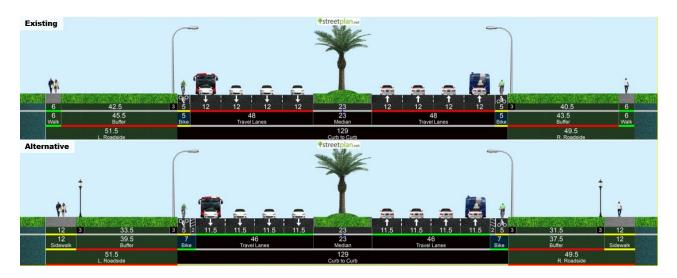
Figure 3. MCS Mixed Traffic Bus Alternative Concept
