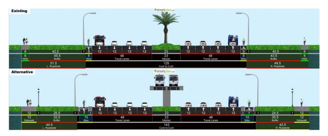
Figure 8. Elevated LRT Alternative Concept
