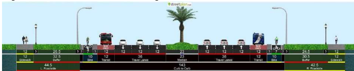
Figure 14. Curbside Dedicated BRT Design Plan
