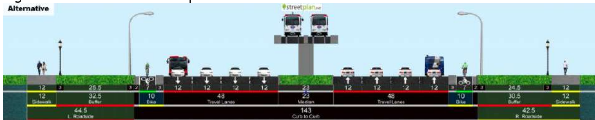
Figure 17. Elevated Grade-Separated LRT
